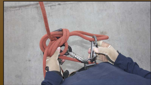
Clip the remaining bight back into your seat harness with another carabiner
