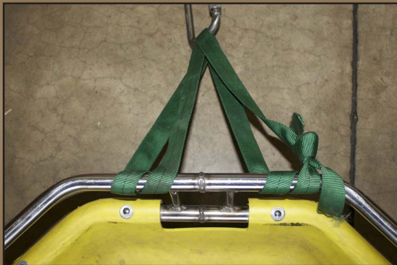
Head Lashing - Wrap an 8' piece of webbing 4 times around the top rail, avoiding the weld then connect to bridle.
