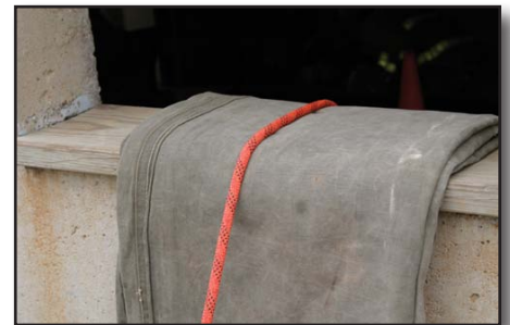
Figure 24-5 A debris carrier can be used for edge protection
