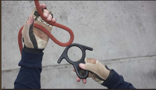
Feed bight of rope down through the 8 plate and back up over the neck
