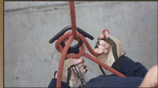
To lock-off, pass the rope behind the 8 plate, around the cleat and back to your right side.
