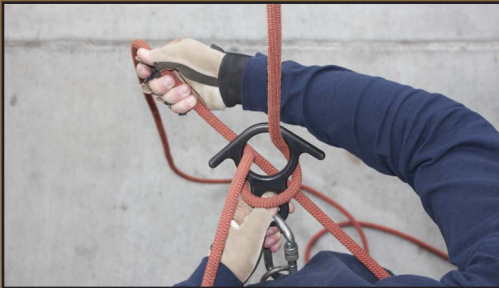
Pass the rope around your left side, along your back, to your right side and prepare to rappel.
